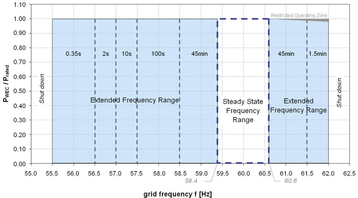
**Figure 2: Extended Frequency Range of REpower MM92 CCV**
